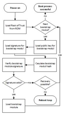
Figure 4. Secure Boot process [3]
