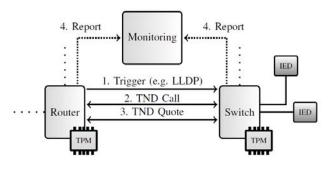
Figure 2. Overview of the Trusted Core Network (TCN)
