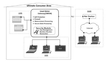
Figure 1. SMGW communication via PLC via the WAN
